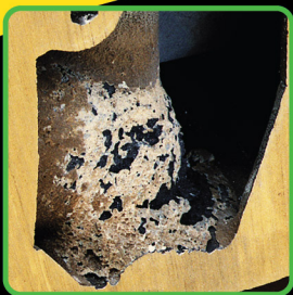
Severe corrosion which can occur when additives that protect the cooling system have been depleted.
