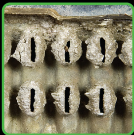
Rust, scale and sludge can plug cooling system fins, preventing proper circulation of coolant.
